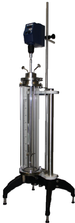
VERDOT Ips 2 PilMod M column w/agitation system (View non contractual)
