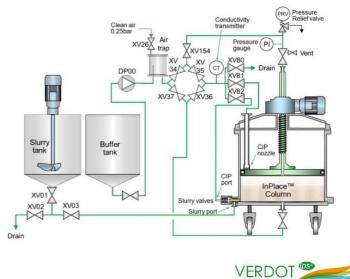
Fig. 2 P&ID of the installation for packing and unpacking
