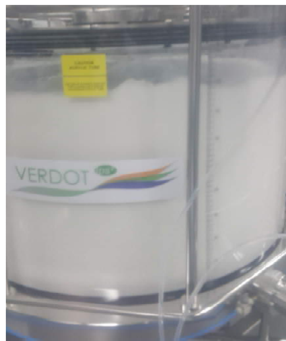
Fig. 6. Re-slurrying with air-sparging .
