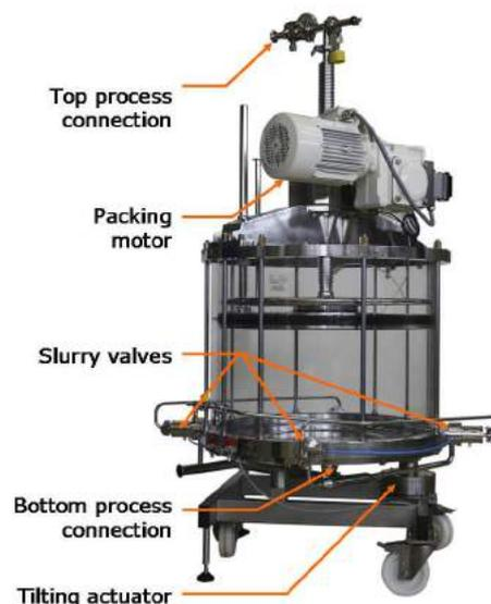
Fig.1. VERDOT Ips<sup>2</sup> InPlace column
