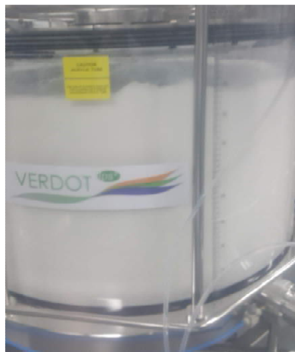
Fig. 6. Re-slurrying with air-sparging .
