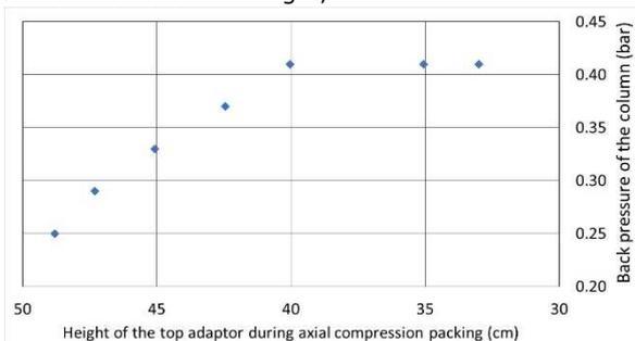
Figure 4 – Back pressure of the column during bed consolidation
