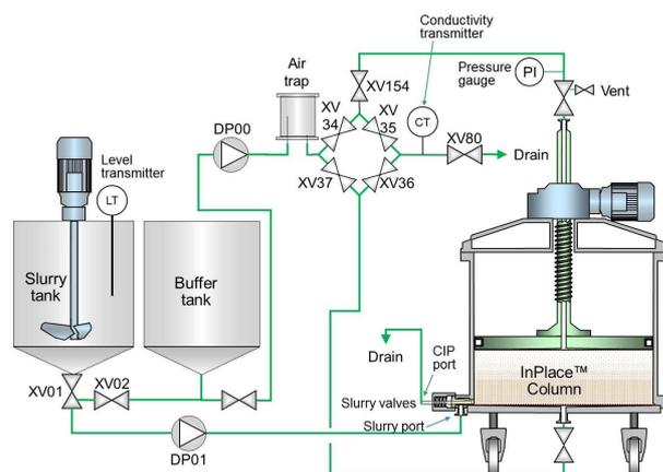
Fig.2. P&ID of the installation
