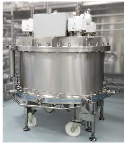
Fig.1. VERDOT InPlace column D160cm with stainless steel tube
