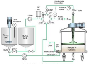
Fig.2. P&ID of the installation
